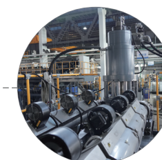
双层储料机头 Double-layer accumulator die head
