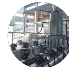
三层储料机头 Triple-layer accumulator die head
